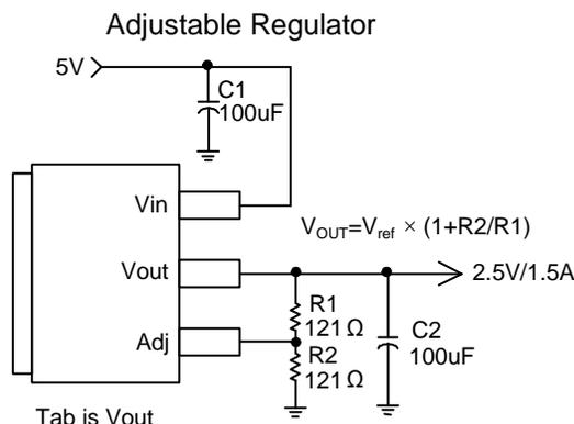
**Note:**  $V_o = V_{RE} * \left( 1 + \frac{R_2}{R_1} \right)$
