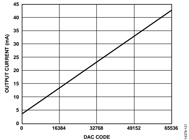
Figure 189. Gain Curve for ANA_FULL_SCALE_CURRENT[9:0] = 1023, DAC Offset = 3.8 mA
