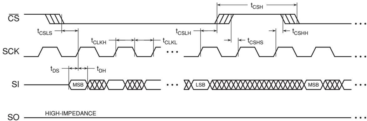
Figure 15-2. Serial Output Timing
