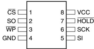
Figure 2-2. 8-UDFN (Top View)
