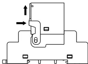
2) Removal of the securing hook is easily performed by releasing the hook and pressing down, as shown in the figure.
