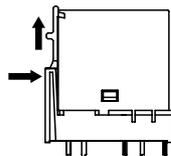
2) Removal of the securing hook is easily performed by releasing the hook and pressing down, as shown in the figure.
