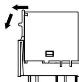
\* To prevent damage and deformity, please use the relay-securing hook at 10 N or less.
