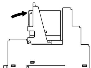
2) Removal of the relay is easily performed by pressing the parts with arrows.
