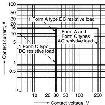
1-(2). Max. switching capacity (2 Form C)
