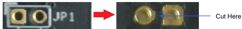
Figure 7. Top and Bottom View of Shorted Jumper. The Bottom View Shows the Trace Location to Cut for Current Measurement
