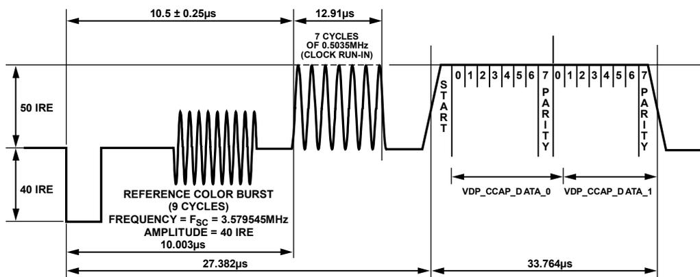
Figure 45. CCAP Waveform and Decoded Data Correlation
