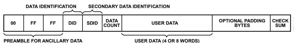
Figure 47. Gemstar and CCAP Embedded Data Packet (Generic)
