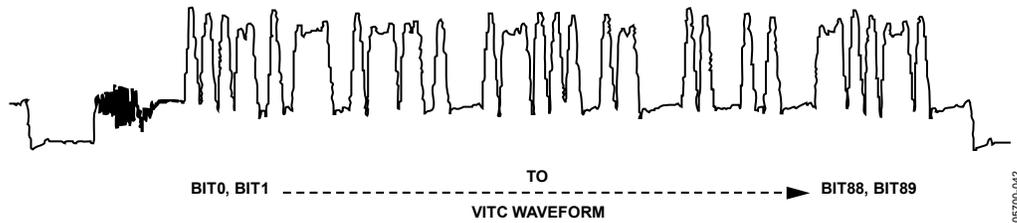
Figure 46. VITC Waveform and Decoded Data Correlation
