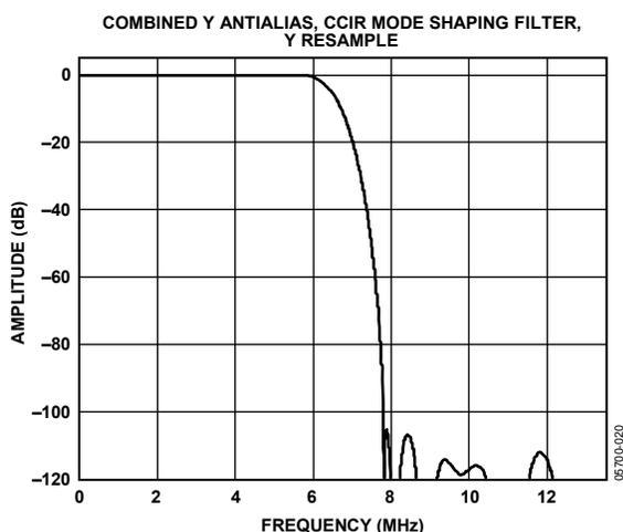
Figure 20. Y S-VHS 18 Extra Wideband Filter (CCIR 601 Compliant)
