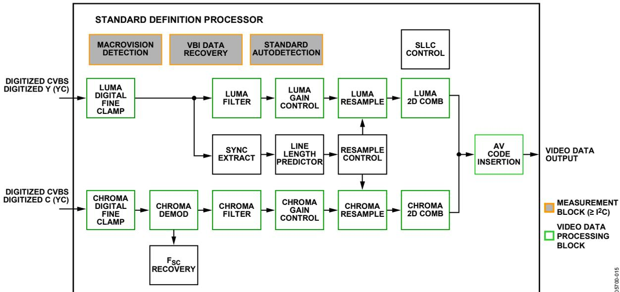
Figure 15. Block Diagram of the Video Processor
