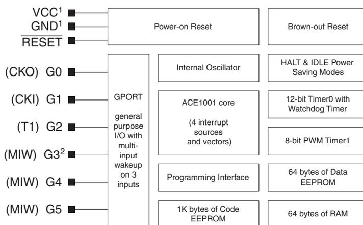
1. 100nf decoupling capacitor recommended.
