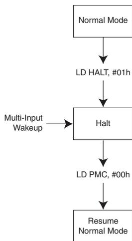
**Figure 29: Recommended IDLE Flow**
