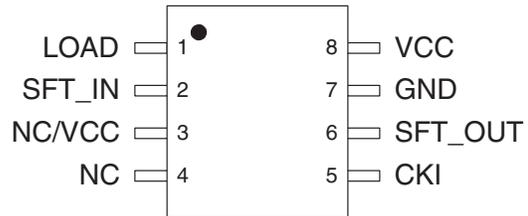
**Figure 3: ACE1001 TSSOP 8-Pin Device Pinout**
