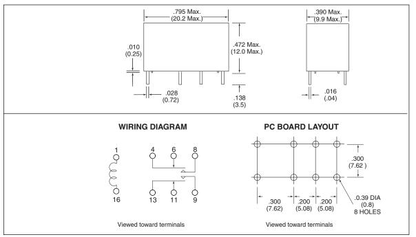
Dimensions in inches with metric equivalents in parentheses. Tolerance: ± .010"
