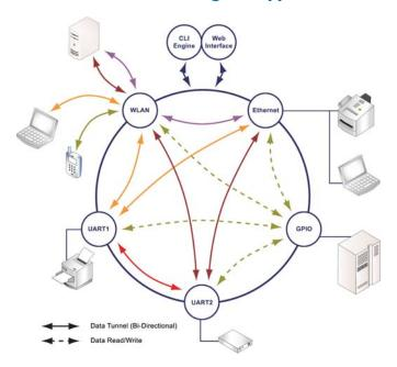
Airborne's unique PortFlex<sup>™</sup> capability enables users to configure communication ports in any combination through a simple setup wizard. Airborne PortFlex<sup>™</sup> supports UART, Ethernet and 802.11 interfaces, and provides the ability to independently configure each port.
