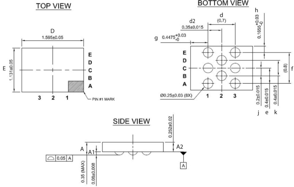
NOTE: BACKSIDE LAMINATE IS INCLUDED IN THE OVERALL DIE THICKNESS DIMENSION.
