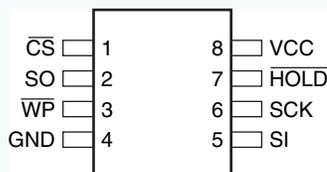
**Figure 2-3. 8-UDFN (Top View)**
