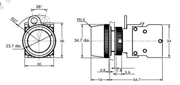
Note: 1. The alternate operation pushbutton is 9.2 mm longer.
