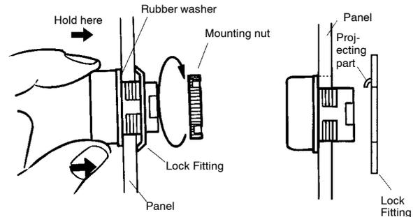
When the panel cutout dimension is 25 mm dia., remove the supplied rubber washer and mount the 25 mm-dia. Ring as shown below. (Since the A22Z-R25 is not attached to the main body, order separately.)
