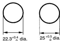
Note: When applying a coating such as paint to a panel, the dimensions should be those after the application of the coating.
