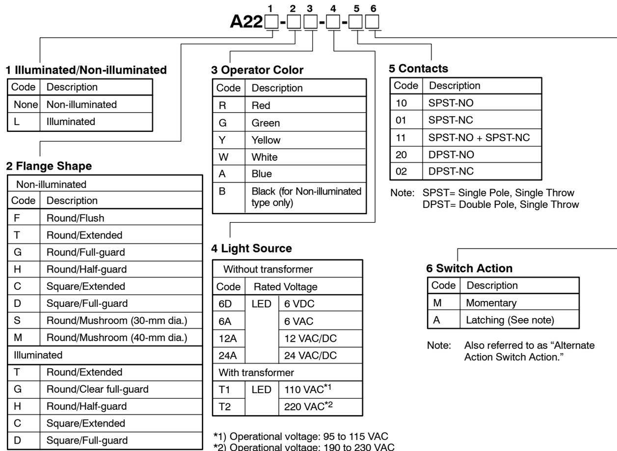
Note: With Transformer types the LED lamp (24 VAC/DC) can be lit by directly applying 110 VAC/DC (220 VAC/DC) to the lamp terminal. The LED is the 24-VAC/DC type.
