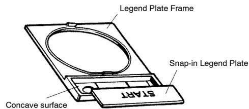
To easily remove the Snap-in Legend Plate from the Legend Plate Frame mounted to the panel, insert a Tool with a thin tip into the space between the Snap-in Legend Plate and the Legend Plate Frame.
