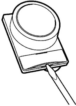
The Snap-in Legend Plate is easily removed by pressing the Snap-in Legend Plate from the back of the Legend Plate Frame.
