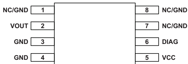
Package LE, 8-Pin eTSSOP Pinouts
