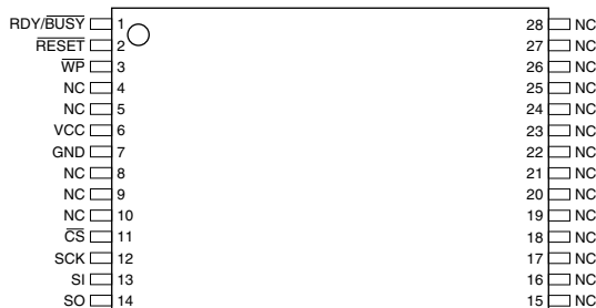
TSOP Top View – Type 1
