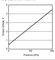
1.-(2) Overall accuracy (Offset voltage) ADP5170 Drive voltage: 5V DC
