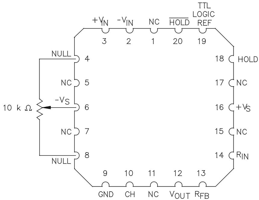
NOTE: For case outline 2, it is recommended that terminals 1 and 11 be connected to ground.
