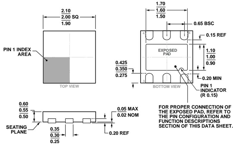
Figure 67. 6-Lead Lead Frame Chip Scale Package [LFCSP\_UD]
