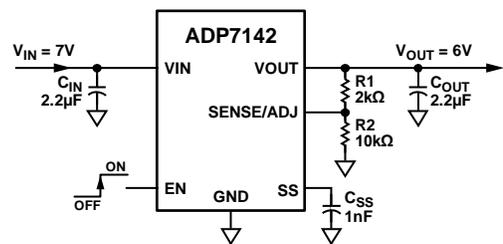
Figure 43. Typical Adjustable Output Voltage Application Schematic
