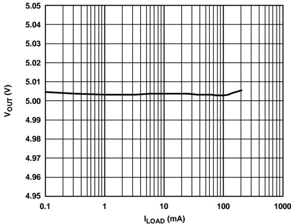
Figure 7. Output Voltage ( $V_{OUT}$ ) vs. Load Current ( $I_{LOAD}$ )
