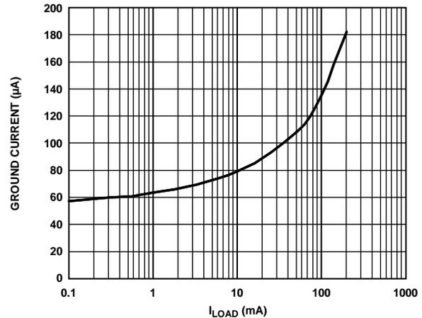
Figure 10. Ground Current vs. Load Current ( $I_{LOAD}$ )
