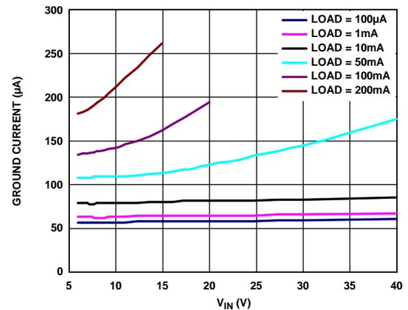
Figure 11. Ground Current vs. Input Voltage ( $V_{IN}$ )
