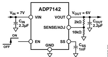
Figure 2. [ADP7142](#) with 5 V Output Adjusted to 6 V
