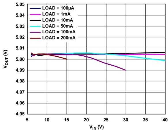
Figure 8. Output Voltage ( $V_{OUT}$ ) vs. Input Voltage ( $V_{IN}$ )
