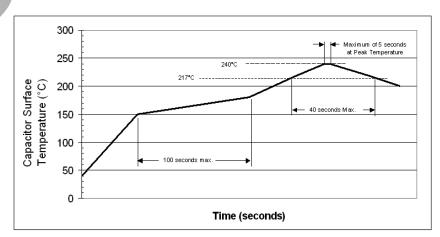
Case sizes 4 thur 6.3 mm dia. should be subjected to just one reflow soldering process. The 8 and 10 mm dia. case sizes should be subjected to a maximum of two reflow soldering processes.
