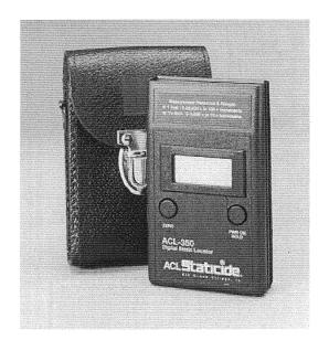
The ACL 350 Digital Static Locator is a non-contact meter that indicates electrostatic field voltage and polarity on charged surfaces. This easy-to-use instrument comes equipped with a Power On/Hold Button and a Zero button.
