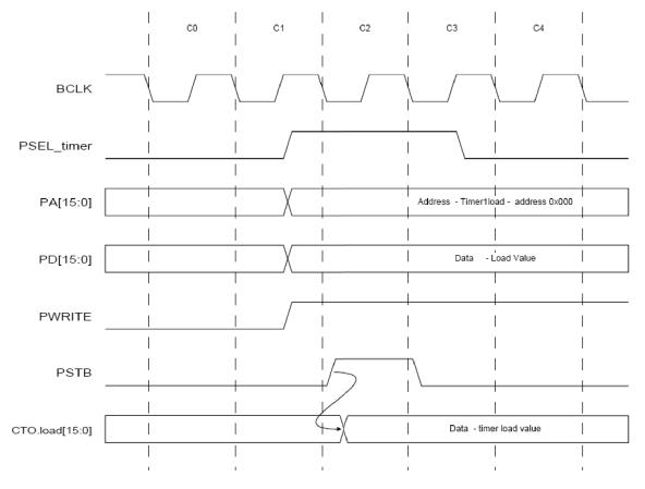
Writes to the Timer module are generated from the Peripheral Bus Controller module. Figure 1-2 summarizes this.
