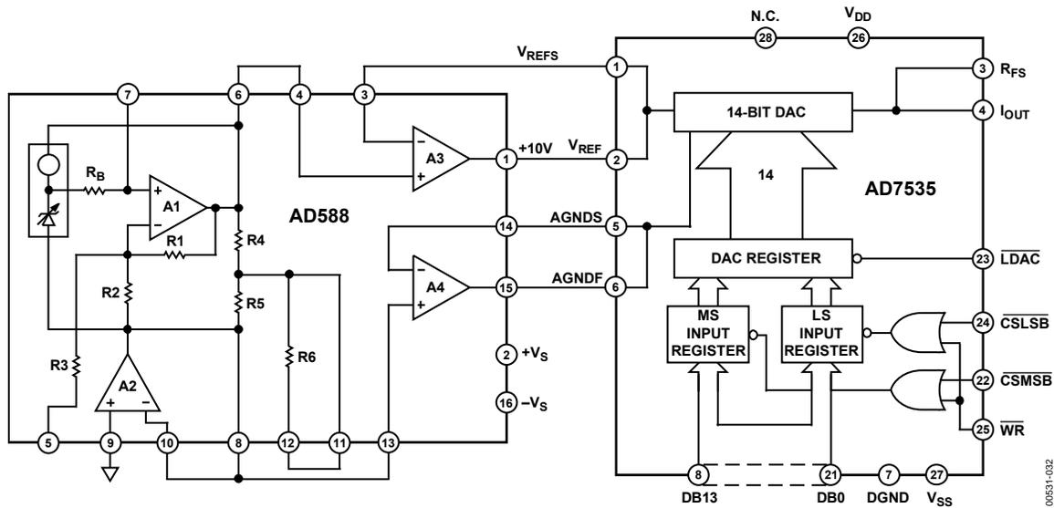
Figure 32. AD588/AD7535 Connections
