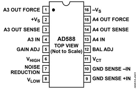
Figure 2. Pin Configuration
