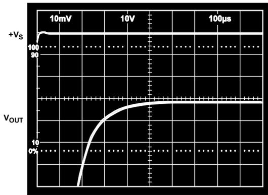
Figure 9. Electrical Turn-On
