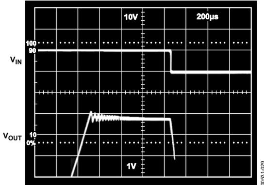
Figure 29. Output Amplifier Step Response,  $C_L = 1 \mu\text{F}$
