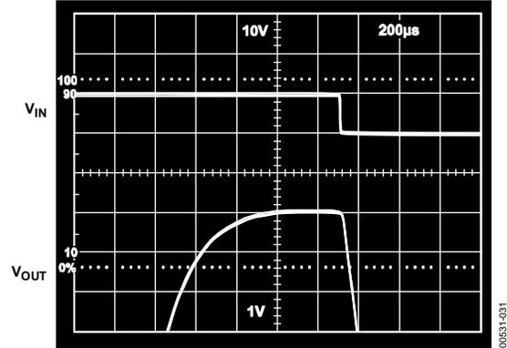
Figure 31. Output Amplifier Step Response Using Figure 30 Compensation
