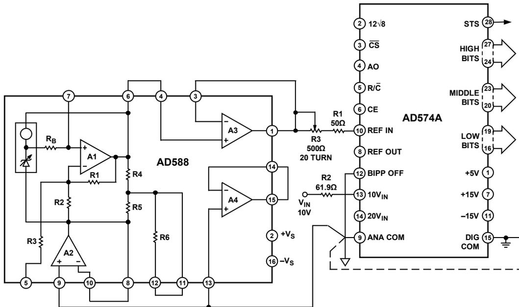
Figure 35. AD588/AD574A Connections
