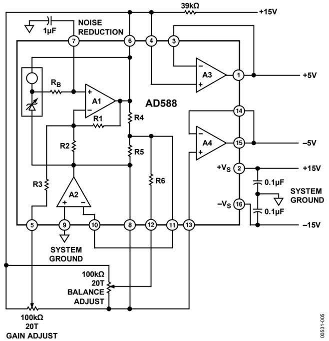
Figure 5. +5 V and -5 V Outputs
