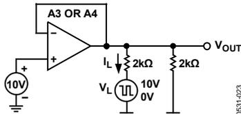
Figure 23. Transient and Constant Load Test Circuit
