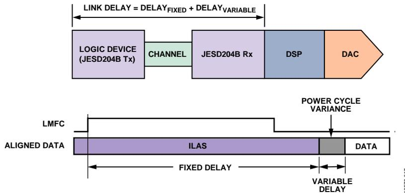
Figure 55. JESD204B Link Delay = Fixed Delay + Variable Delay
