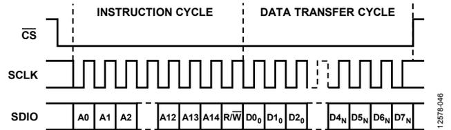
Figure 40. Serial Register Interface Timing, LSB First, ADDRINC = 1
