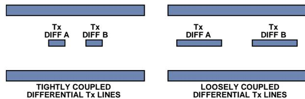
Figure 69. Tightly Coupled vs. Loosely Coupled Differential Traces
