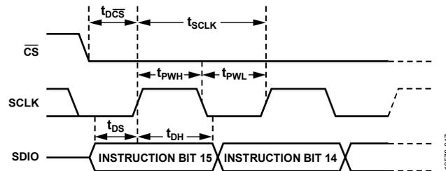
Figure 42. Timing Diagram for Serial Port Register Write
