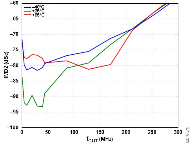
Figure 88. Postcalibration IMD2 over Temperature, Calibrated at 25°C
