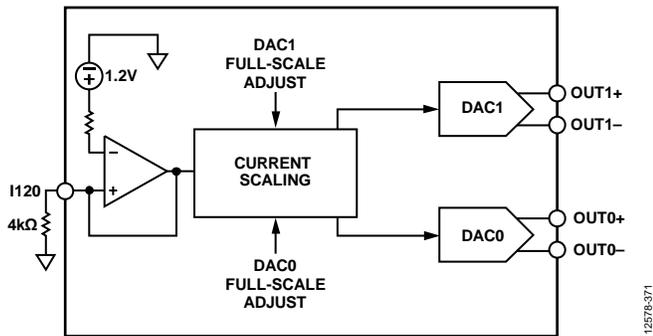
Figure 81. Simplified Block Diagram of DAC Core
