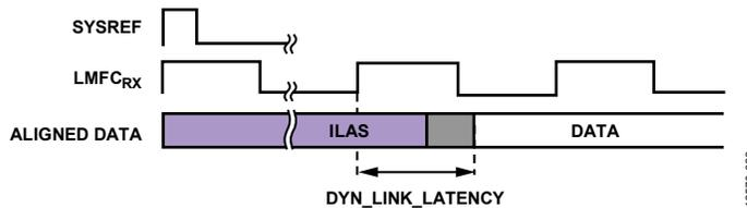
Figure 57. DYN\_LINK\_LATENCY Illustration
