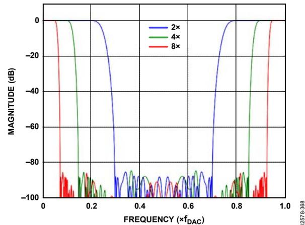
Figure 72. All Band Responses of Interpolation Filters
