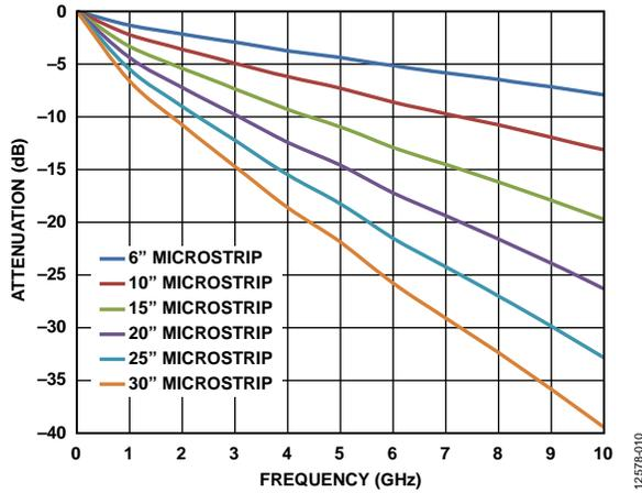
Figure 49. Insertion Loss of 50Ω Microstrips on FR-4
