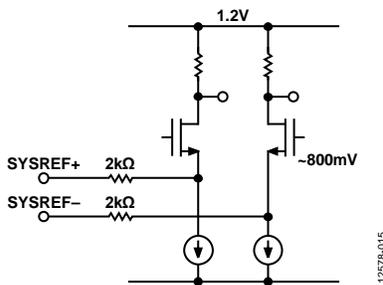
Figure 52.  $\text{SYSREF}_{\pm}$  Input Circuit
