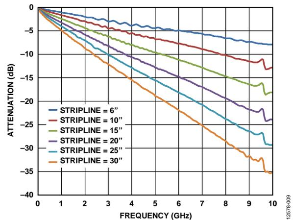
Figure 48. Insertion Loss of 50 Ohm Striplines on FR-4
