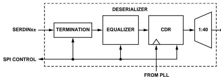
Figure 45. Deserializer Block Diagram
