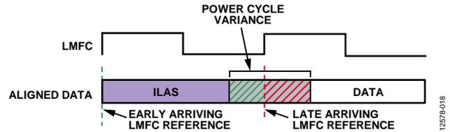
Figure 53. Link Delay > LMFC Period Example
