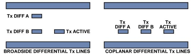
Figure 68. Broadside vs. Coplanar Differential Stripline Routing Techniques
