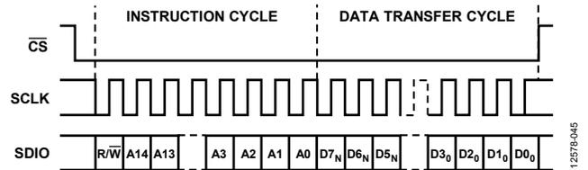
Figure 39. Serial Register Interface Timing, MSB First, ADDRINC = 0
