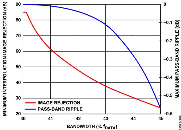
Figure 73. Interpolation Filter Performance Beyond Specified Bandwidth
