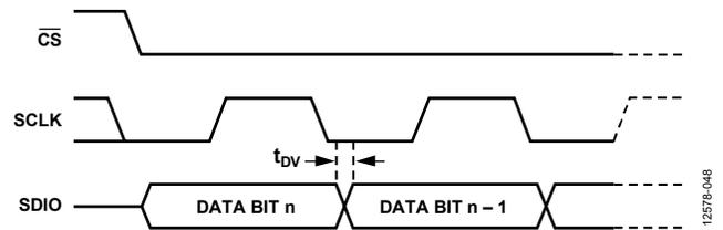
Figure 41. Timing Diagram for Serial Port Register Read
