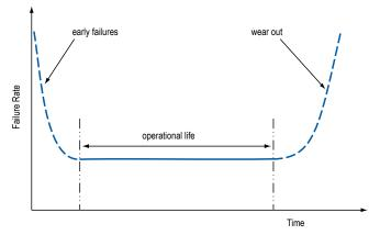
The failure rate is derived from our periodic test results. The failure rate ( $\lambda_R$ ) is, therefore, only given at test temperature for life tests. An estimation is also given at 60°C.
