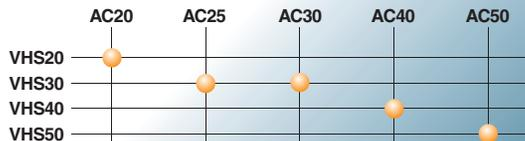
An interface part is required if a spacer or spacer with bracket shown in the table below is attached to a modular FRL.
