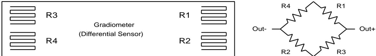
Because all four bridge resistors contribute to the sensor's output, at maximum differential field NVE's gradiometers can provide double the output signal of our magnetometer parts—approximately 700 mV with a 5V supply. In practice, the gradient fields are typically not high enough to give this maximum signal, but signal levels of 50 mV to 200 mV are common.
