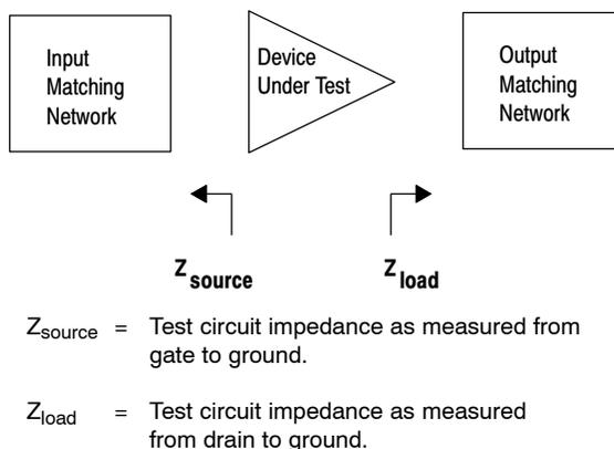
**Figure 3. Data Sheet Impedance Format for Single-Ended Devices**
