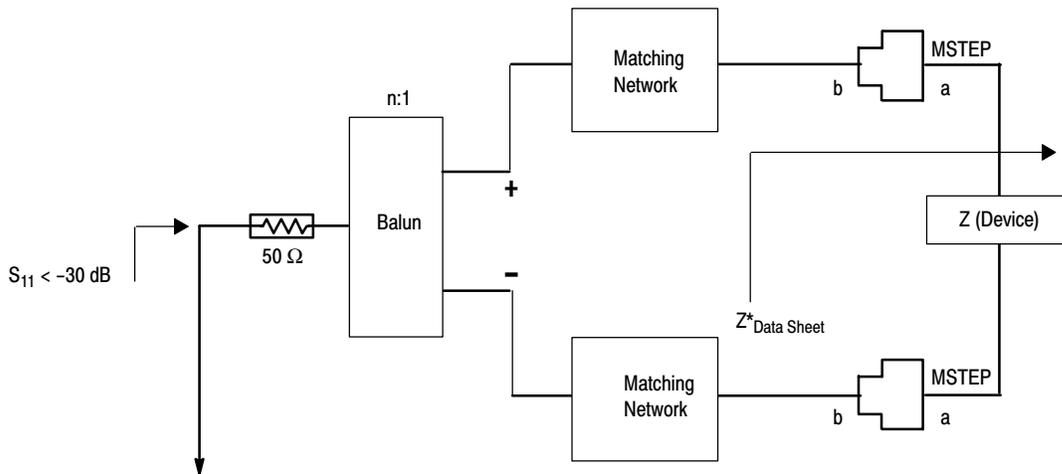
Figure 11. Generalized Schematic Used to Optimize Matching Network
