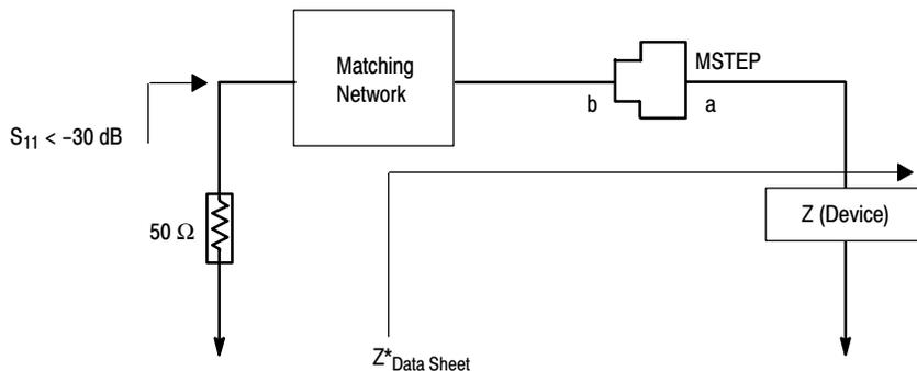
**Figure 6. Generalized Schematic Used to Optimize Matching Network**
