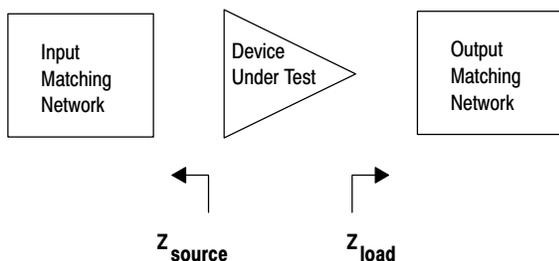
**Figure 4. Optimal Impedances for an MRF19125 Test Fixture**
