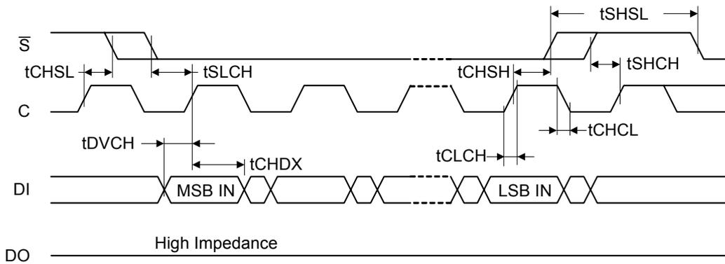
**Figure 29. Write Protect Setup and Hold Timing during WRSR when (SRP1, SRP0) = (0, 1)**
