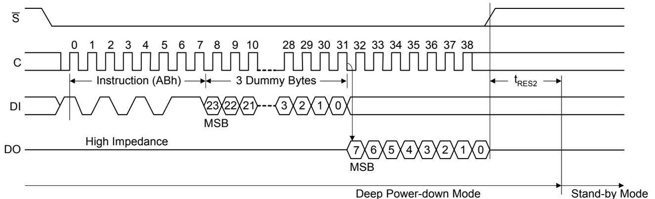
Note: The value of the 8-bit Electronic Signature, for A25L032 is 15h.
