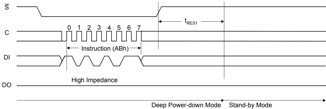
Driving Chip Select ( $\overline{S}$ ) High after the 8-bit instruction byte has been received by the device, but before the whole of the 8-bit Electronic Signature has been transmitted for the first time (as shown in Figure 23.), still insures that the device is put into Stand-by Power mode. If the device was not previously in the Deep Power-down mode, the transition to the Stand-by Power mode is immediate. If the device was
