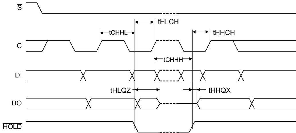
**Figure 31. Output Timing**
