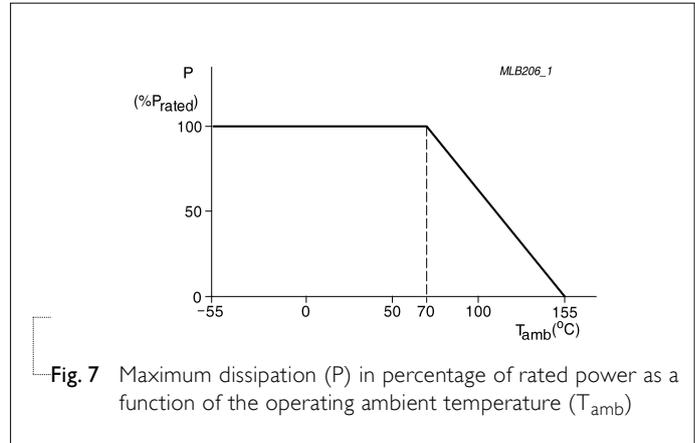
Fig. 7 Maximum dissipation (P) in percentage of rated power as a function of the operating ambient temperature (T<sub>amb</sub>)
