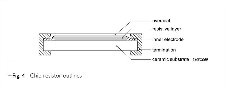
Fig. 4 Chip resistor outlines
