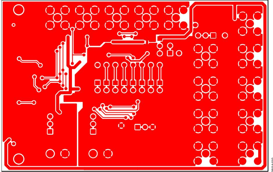
Figure 9. Solder Side PCB Drawing
