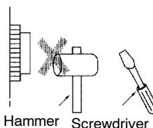
Do not operate the Switch with hard or sharp objects.
