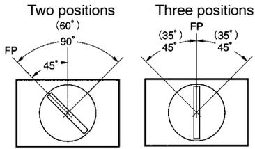
Note: The angle used for automatic reset is shown in parentheses.
