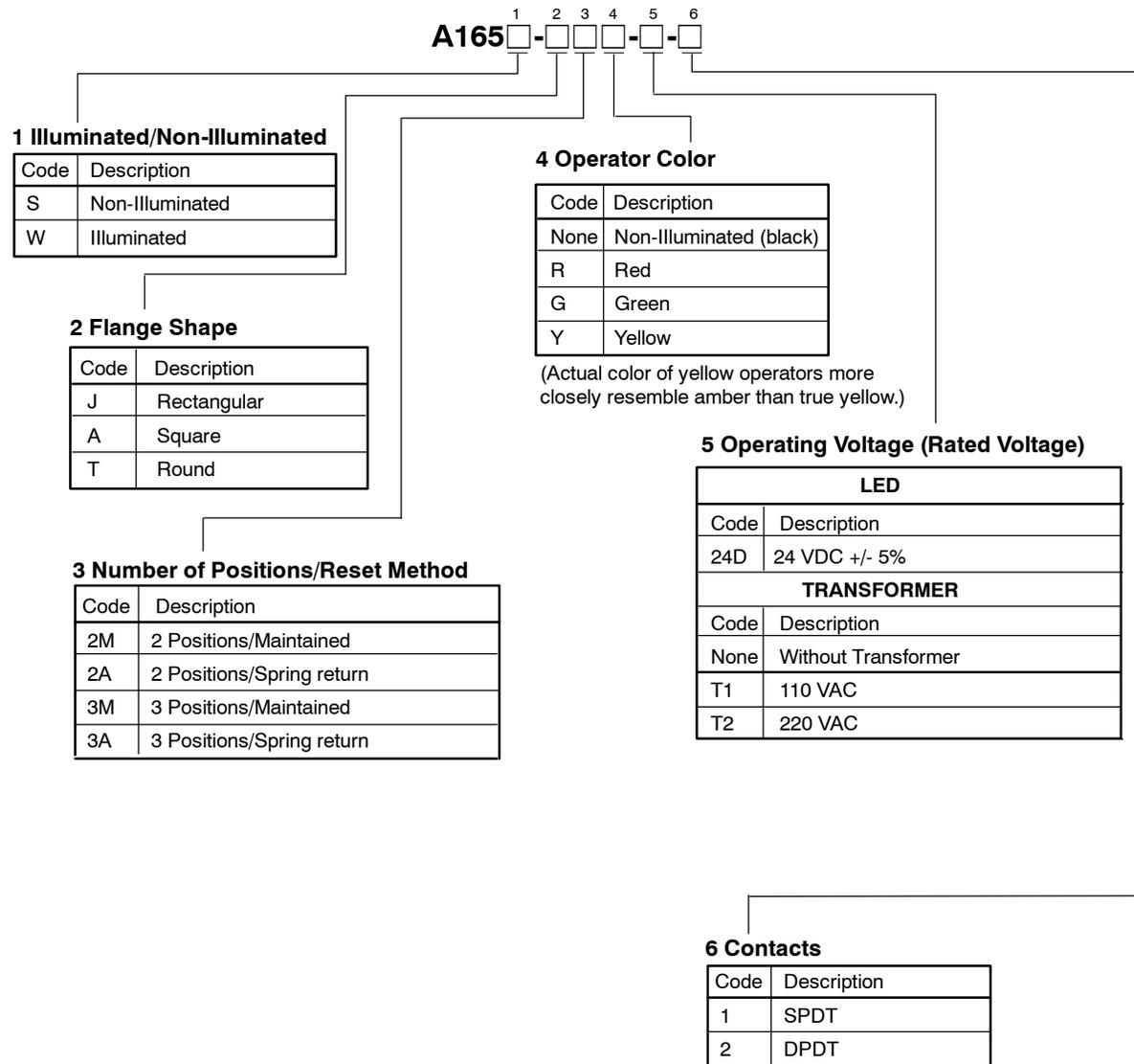
■ PART NUMBERS: A165S ASSEMBLED NON-ILLUMINATED KNOB-TYPE SELECTOR SWITCH
