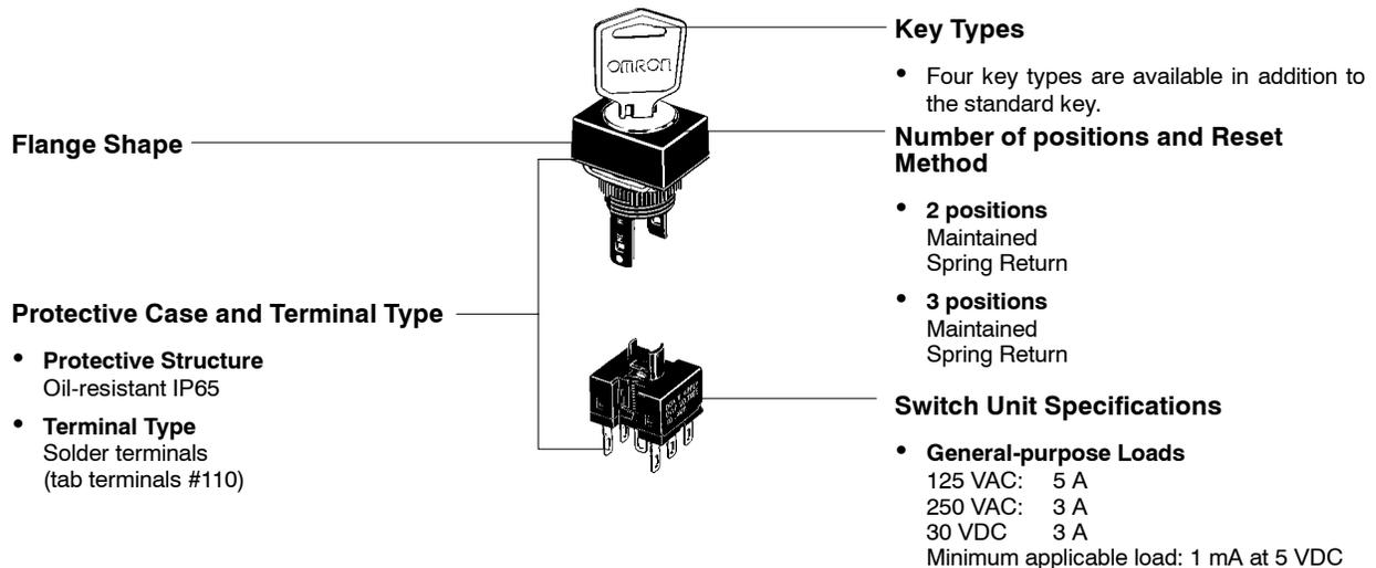
**■ PART NUMBER NOMENCLATURE A165K ASSEMBLED KEY-TYPE SELECTOR SWITCH (COMPLETE ASSEMBLY)**
