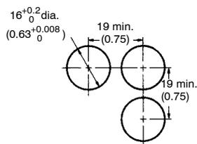
Note: 1. Make sure the thickness of the mounting panel is between 0.5 and 3.2 mm. If, however, a Switch Guard or Dust Cover is used, the thickness of the mounting panel must be between 0.5 and 2 mm.
