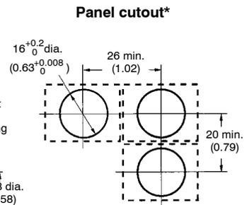
Note: Plate thickness of the panel should be 1.0 to 3.2 mm.
