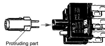
The Lamp can be mounted from the operating part end by using the A16Z-5080 Extractor. The lamp can be mounted by following the opposite procedure for removing the Lamp.
