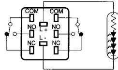
Note: The L+ is not shown on the Switch Unit.
