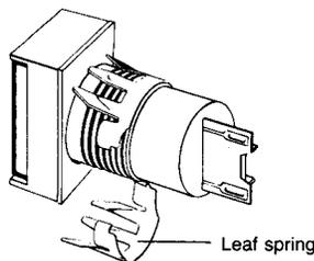
Insert the buzzer assembly into the hole on the mounting panel from the front.
