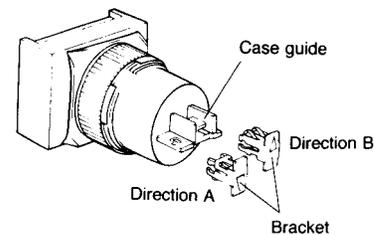
To produce continuous sounds, attach the bracket to the case guide so that the triangle on the bracket faces direction B.
