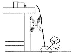
Do not allow the Switch to drop and hit the ground.
