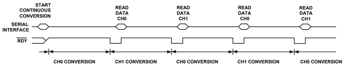
Figure 19. Continuous Conversion, CH0 and CH1,  $\overline{\text{RDYFN}} = 0$
