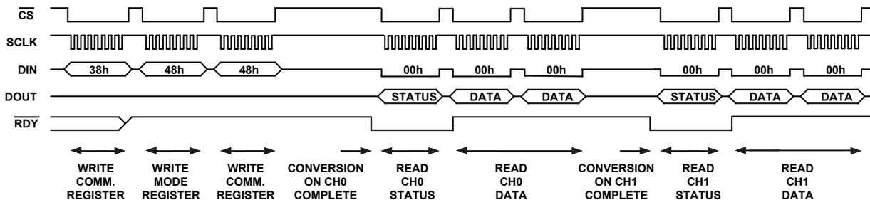
Figure 22. Continuous Conversion, CH0 and CH1, Continuous Read
