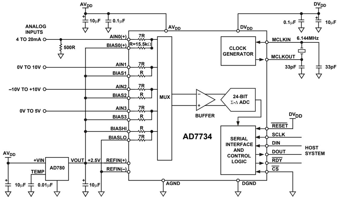
Figure 29. Typical Connections for the AD7734 Application
