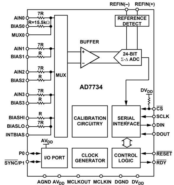
Figure 12. Block Diagram
