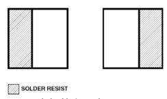
Figure 8. Recommended soldering pad pattern.
