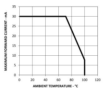
Figure 4. Maximum forward current vs. ambient temperature. Derated based on  $T_{J\,MAX}$  = 110°C,  $R_{\theta\,JA}$  = 500°C/W.
