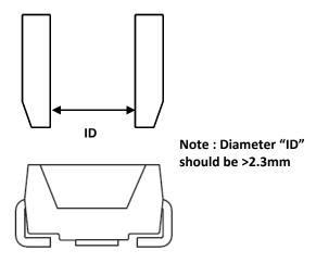
Figure 7. Recommended Pick and Place Nozzle Size
