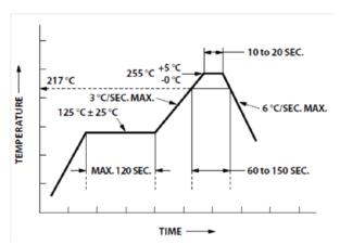
Figure 6. Recommended Pb-free reflow soldering profile.
