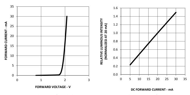
Figure 2. Forward current vs. forward voltage
