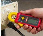
The non-contact voltage (NCV) function checks for voltage presence.
