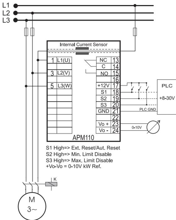
Fig.4 Typical connection with internal sensor
