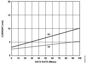
Figure 10. Typical ADuM1280 or ADuM1285 V<sub>DD2</sub> Supply Current vs. Data Rate for 5 V and 3 V Operation
