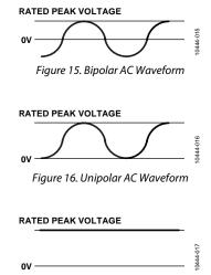
Figure 17. DC Waveform
