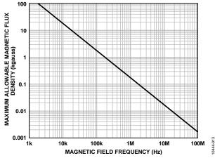
Figure 13. Maximum Allowable External Magnetic Flux Density
