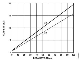
Figure 9. Typical ADuM1280 or ADuM1285  $V_{\text{DD1}}$  Supply Current vs. Data Rate for 5 V and 3 V Operation
