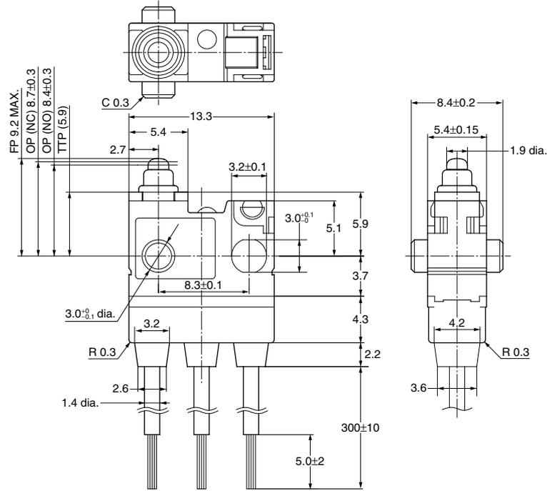
\* Wire lead thickness : 0.3mm<sup>2</sup>
