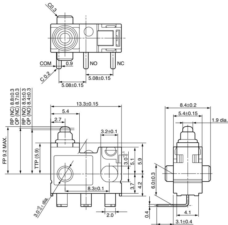
4. Wire leads bottom type: Mounting hole 3mm, standard type
