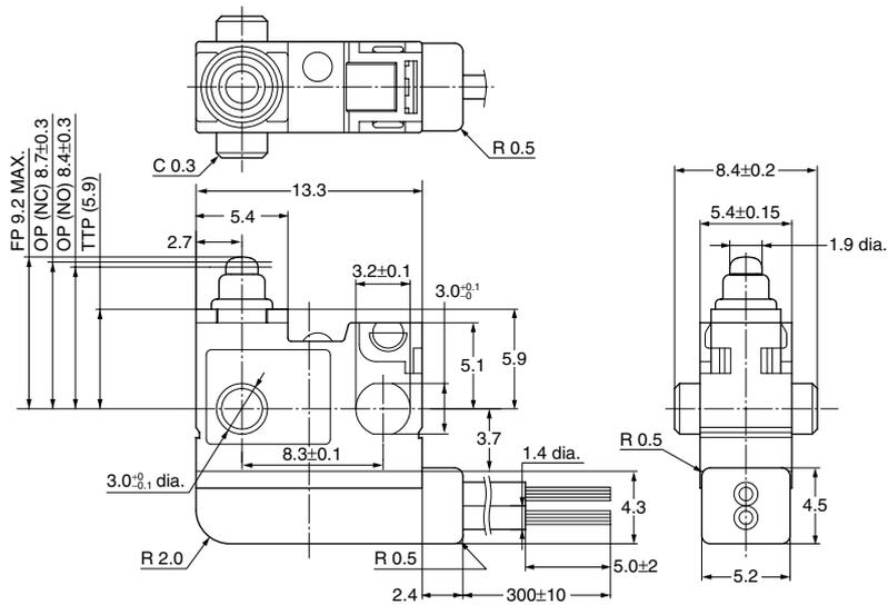
\* Wire lead thickness : 0.3mm<sup>2</sup>
