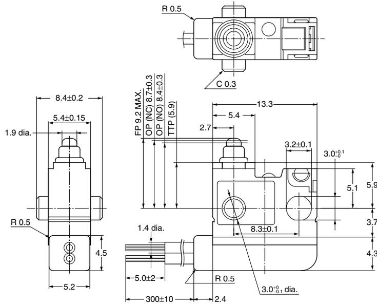
\* Wire lead thickness : 0.3mm<sup>2</sup>
