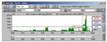
The Execution Profile graph allows to identify procedures that are executed frequently so that they can be optimized to gain system performance.
