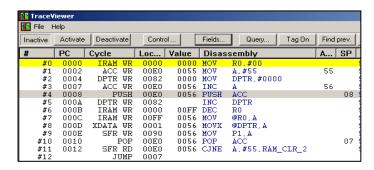
All IRAM, XFR and XDATA transactions in trace contain the Value read or written and the address. A separate columns for Accumulator (A) and Stack Pointer (SP) show the exact values as soon as they are changed.
