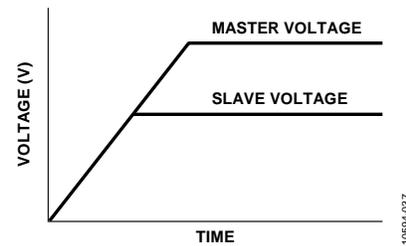
Figure 31. Coincident Tracking
