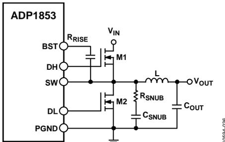
Figure 30. Application Circuit with a Snubber
