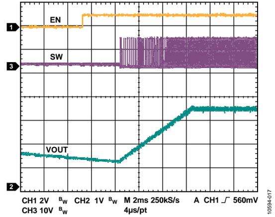
Figure 13. Soft Start with Precharged Output, 3.3 V<sub>OUT</sub> Forced PWM
