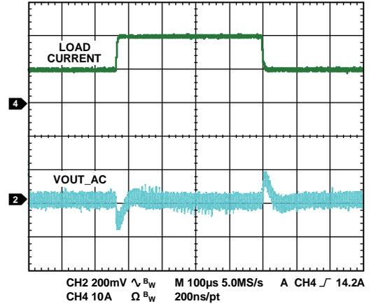
Figure 8. 10 A to 20 A Load Step,
