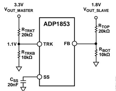
Figure 32. Example of a Coincident Tracking Circuit
