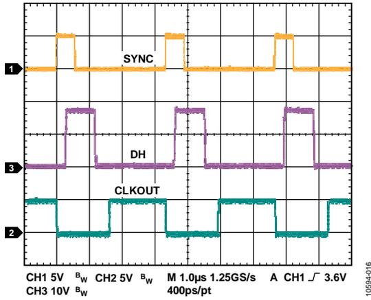
Figure 10. Synchronization and CLKOUT,  $f_{SYNC} = 300$  kHz
