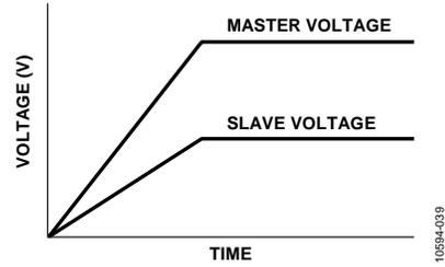
Figure 33. Ratiometric Tracking
