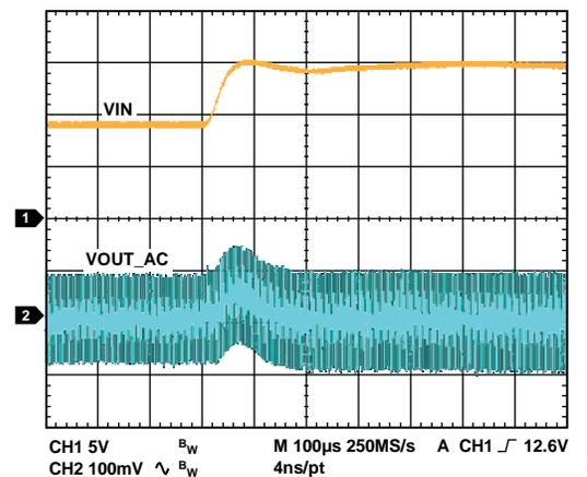
Figure 9. 9 V to 15 V Line Step,
