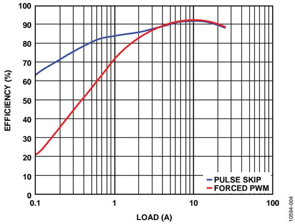
Figure 4. Efficiency Plot
