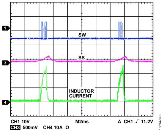
Figure 22. Current-Limit Hiccup Mode, 20 A Current Limit
