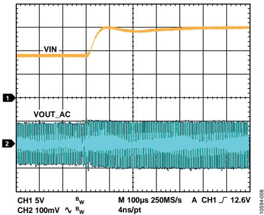
Figure 6. 9 V to 15 V Line Step,
