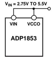
Figure 20. Configuration for  $V_{IN} < 5.5 V$
