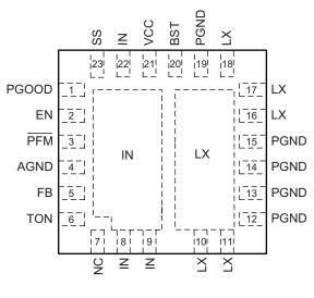
23-Pin 4mm x 4mm QFN (Top View)
