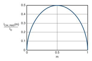
Figure 3. I<sub>CIN</sub> vs. Voltage Conversion Ratio
