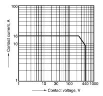
2. Max. switching power (DC resistive load)
