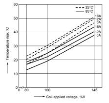
1-2. Coil temperature rise (200mW type) Sample: ALE74B12, 6 pcs. Point measured: coil inside
