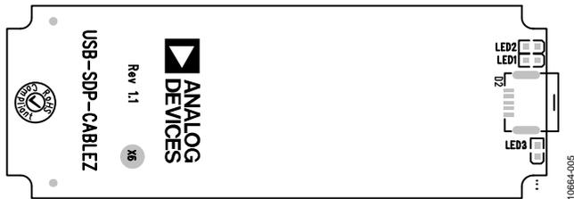
Figure 5. USB-SDP-CABLEZ Board LEDs
