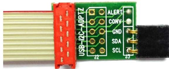
Figure 3. USB-I2C-ADPTZ Adapter Board
