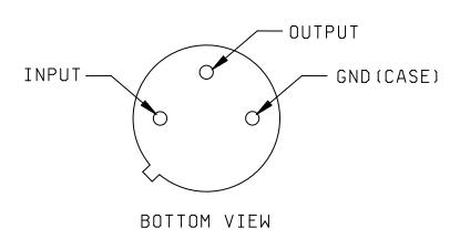
FIGURE 2. <u>Terminal connections</u>.
