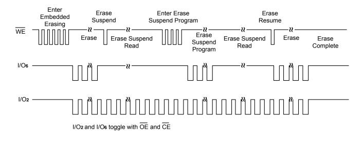
Note : Both I/O<sub>6</sub> and I/O<sub>2</sub> toggle with OE or CE. See the text on I/O<sub>8</sub> and I/O<sub>2</sub> in the section "Write Operation Statue" for more information.
