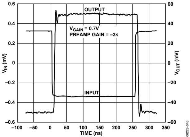
Figure 46. Inverting Gain Small-Signal Pulse Response (See Figure 70)
