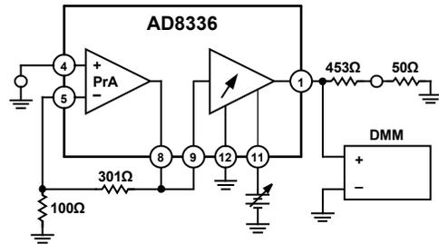
Figure 60. Offset Voltage
