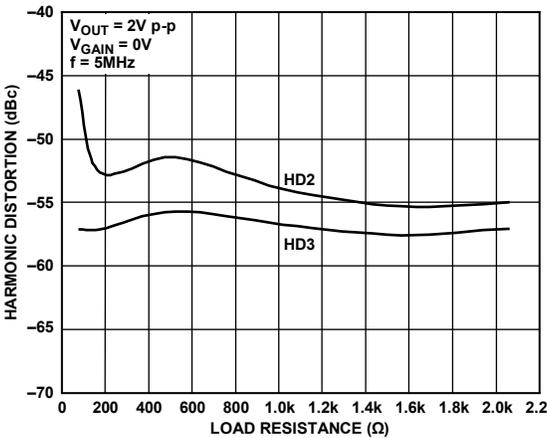
Figure 35. Harmonic Distortion vs. Load Resistance (See Figure 64)
