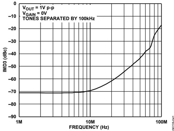
Figure 41. IMD3 vs. Frequency (see Figure 76)
