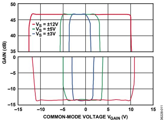
Figure 11. Gain vs. Common-Mode Voltage at  $V_{GAIN}$
