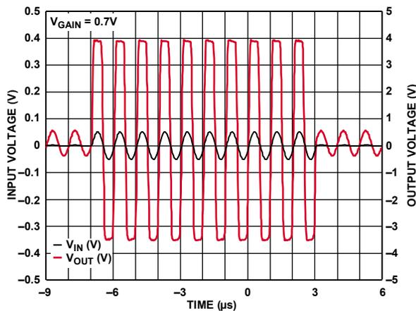
Figure 53. VGA Overdrive Recovery (See Figure 67)
