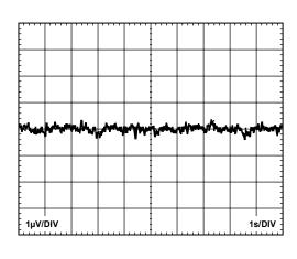
Figure 9. 0.1 Hz to 10 Hz RTI Voltage Noise (G = 1000)
