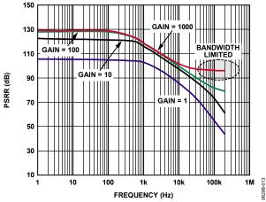
Figure 11. Positive PSRR vs. Frequency, RTI
