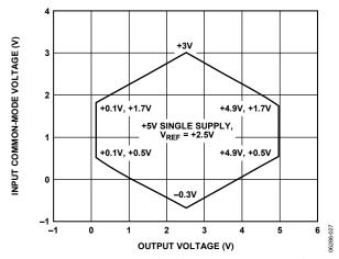
Figure 25. Input Common-Mode Voltage Range vs. Output Voltage, G = 1,  $V_S = 5$  V,  $V_{REF} = 2.5$  V
