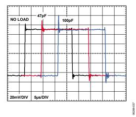
Figure 35. Small Signal Pulse Response for Various Capacitive Loads,  $V_S = \pm 15 V$ ,  $V_{REF} = 0 V$
