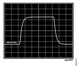
Figure 48. Small Signal Pulse Response, G=100,  $R_{\text{LOAD}}=2$  k $\Omega$ ,  $C_{\text{LOAD}}=100$  pF,  $V_{\text{S}}=5$  V,  $V_{\text{REF}}=2.5$  V
