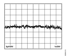
Figure 8. 0.1 Hz to 10 Hz RTI Voltage Noise (G = 1)
