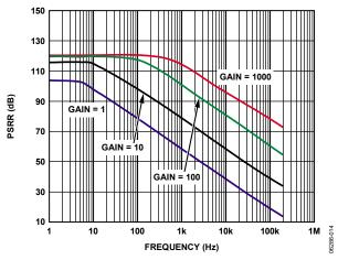
Figure 12. Negative PSRR vs. Frequency, RTI
