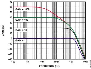
Figure 19. Gain vs. Frequency
