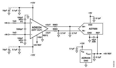
Figure 64. Driving a Differential ADC
