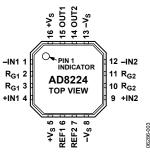
Figure 3. Pin Configuration
