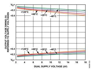
Figure 30. Output Voltage Swing vs. Dual Supply Voltage,  $R_{LOAD} = 10 \text{ k}\Omega$ , G = 10,  $V_{REF} = 0 \text{ V}$
