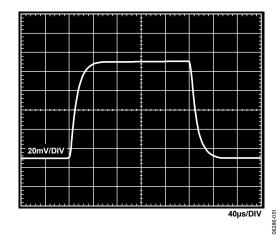
Figure 49. Small Signal Pulse Response, G=1000,  $R_{LOAD}=2$   $k\Omega$ ,  $C_{LOAD}=100$  pF,  $V_S=5$  V,  $V_{REF}=2.5$  V
