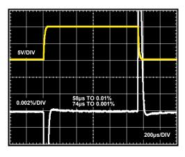
Figure 41. Large Signal Pulse Response and Settle Time, G=1000,  $R_{LOAD}=10~k\Omega,~V_S=\pm15~V,~V_{REF}=0~V$
