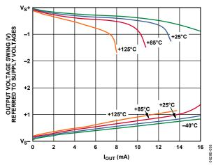
Figure 34. Output Voltage Swing vs. Output Current,  $V_S = 5 V$ ,  $V_{REF} = 2.5 V$
