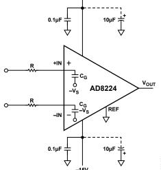
Figure 59. RFI Filtering Without External Capacitors
