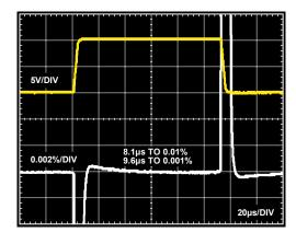
Figure 40. Large Signal Pulse Response and Settle Time, G=100,  $R_{LOAD}=10$  k $\Omega$ ,  $V_{S}=\pm15$  V,  $V_{REF}=0$  V
