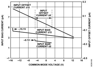
Figure 13. Input Bias Current and Input Offset Current vs. Common-Mode Voltage
