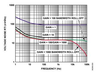
Figure 7. Voltage Spectral Density vs. Frequency
