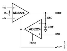
Figure 62. Differential Circuit Schematic
