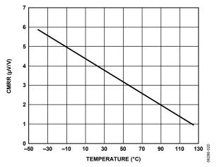
Figure 18. Change in CMRR vs. Temperature, G = 1
