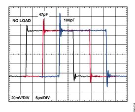
Figure 36. Small Signal Pulse Response for Various Capacitive Loads,  $V_S = 5 V$ ,  $V_{REF} = 2.5 V$
