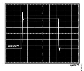
Figure 42. Small Signal Pulse Response, G=1,  $R_{LOAD}=2$  k $\Omega$ ,  $C_{LOAD}=100$  pF,  $V_S=\pm15$  V,  $V_{REF}=0$  V
