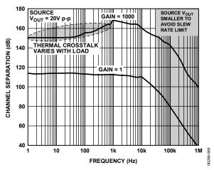
Figure 52. Channel Separation vs. Frequency,  $R_{LOAD}=2~k\Omega$ , Source Channel at G=1
