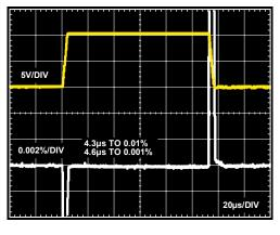
Figure 39. Large Signal Pulse Response and Settle Time, G = 10,  $R_{LOAD}$  = 10 k $\Omega$ ,  $V_{S}$  =  $\pm$ 15 V,  $V_{REF}$  = 0 V
