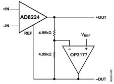
Figure 63. Differential Output Using Op Amp
