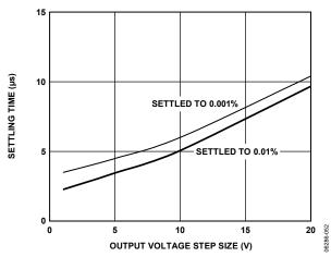
Figure 50. Settling Time vs. Output Voltage Step Size,  $(G = 1) \pm 15 V$ ,  $V_{REF} = 0 V$
