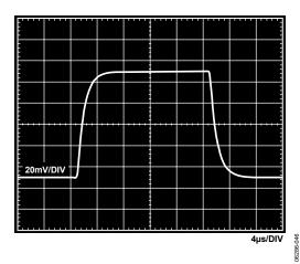
Figure 44. Small Signal Pulse Response, G=100,  $R_{LOAD}=2$  k $\Omega$ ,  $C_{LOAD}=100$  pF,  $V_S=\pm15$  V,  $V_{REF}=0$  V
