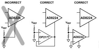
Figure 56. Driving the Reference Pin
