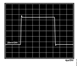
Figure 43. Small Signal Pulse Response, G=10,  $R_{LOAD}=2$  k $\Omega$ ,  $C_{LOAD}=100$  pF,  $V_{S}=\pm15$  V,  $V_{REF}=0$  V
