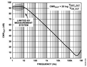
Figure 54. Differential Output Configuration: Common-Mode Output (CMR<sub>OUT</sub>) vs. Frequency
