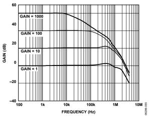
Figure 53. Differential Output Configuration: Gain vs. Frequency
