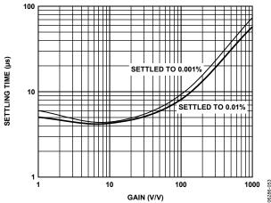
Figure 51. Settling Time vs. Gain for a 10 V Step,  $V_S = \pm 15 V$ ,  $V_{REF} = 0 V$
