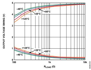
Figure 32. Output Voltage Swing vs. Load Resistance,  $V_S = 5 V$ ,  $V_{REF} = 2.5 V$
