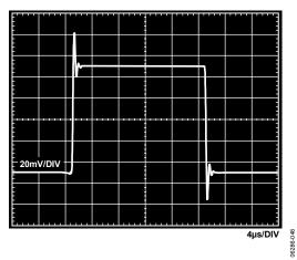
Figure 46. Small Signal Pulse Response, G=1,  $R_{LOAD}=2$  k $\Omega$ ,  $C_{LOAD}=100$  pF,  $V_S=5$  V,  $V_{REF}=2.5$  V
