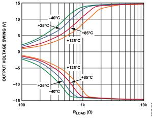
Figure 31. Output Voltage Swing vs. Load Resistance,  $V_S = \pm 15 \text{ V}$ ,  $V_{REF} = 0 \text{ V}$
