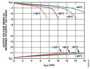
Figure 33. Output Voltage Swing vs. Output Current,  $V_S = \pm 15 \text{ V}$ ,  $V_{REF} = 0 \text{ V}$
