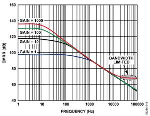
Figure 17. CMRR vs. Frequency, 1 k $\Omega$  Source Imbalance
