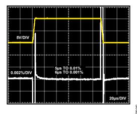
Figure 38. Large Signal Pulse Response and Settle Time, G=1,  $R_{LOAD}=10~k\Omega,~V_S=\pm15~V,~V_{REF}=0~V$
