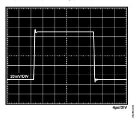
Figure 47. Small Signal Pulse Response, G=10,  $R_{LOAD}=2$  k $\Omega$ ,  $C_{LOAD}=100$  pF,  $V_S=5$  V,  $V_{REF}=2.5$  V
