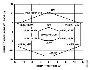
Figure 26. Input Common-Mode Voltage Range vs. Output Voltage, G = 100,  $V_{REF} = 0$  V
