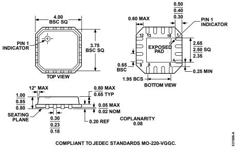
Figure 66. 16-Lead Lead Frame Chip Scale Package [LFCSP\_VQ] 4 mm × 4 mm Body, Very Thin Quad (CP-16-13) Dimensions are shown in millimeters
