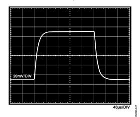
Figure 45. Small Signal Pulse Response,  $G=1000,\,R_{LOAD}=2\,k\Omega,\,C_{LOAD}=100\,pF,\,V_S=\pm15\,V,\,V_{REF}=0\,V$
