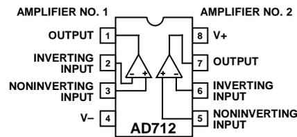
Figure 1. 8-Lead PDIP (N-Suffix),
