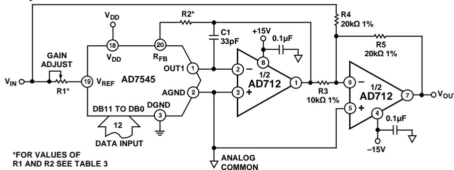
Figure 40. Bipolar Operation
