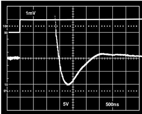
Figure 41. Positive Settling Characteristics for AD712 with AD7545
