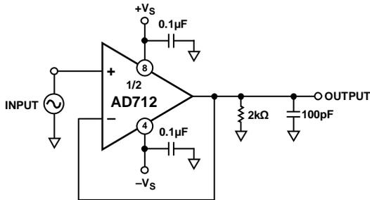
Figure 21. THD Test Circuit
