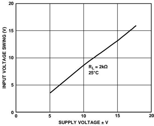
Figure 2. Input Voltage Swing vs. Supply Voltage
