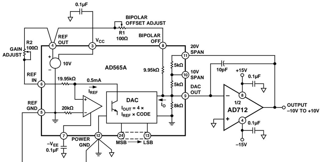
Figure 31. ±10 V Voltage Output Bipolar DAC
