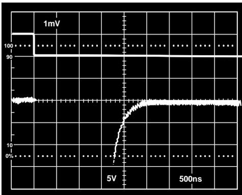
Figure 42. Negative Settling Characteristics for AD712 with AD7545
