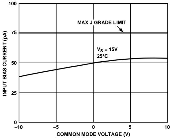
Figure 8. Input Bias Current vs. Common-Mode Voltage
