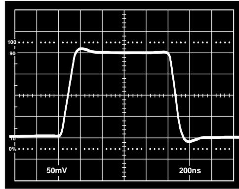
Figure 28. Unity-Gain Inverter Pulse Response (Small Signal)
