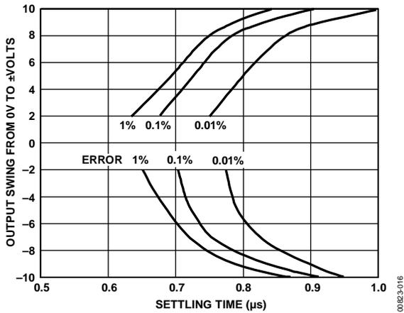
Figure 16. Output Swing and Error vs. Settling Time
