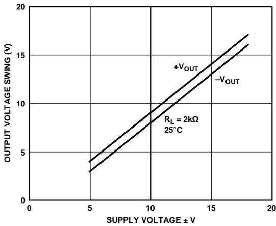
Figure 3. Output Voltage Swing vs. Supply Voltage
