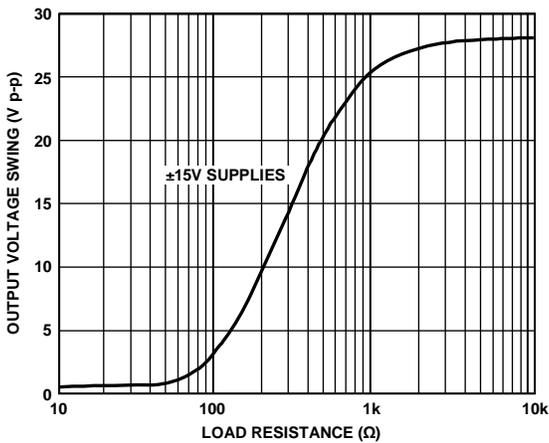
Figure 4. Output Voltage Swing vs. Load Resistance
