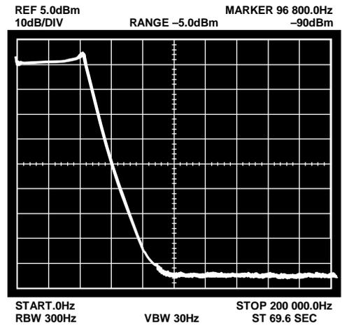
Figure 52. High Frequency Response for 9-Pole Chebyshev Filter
