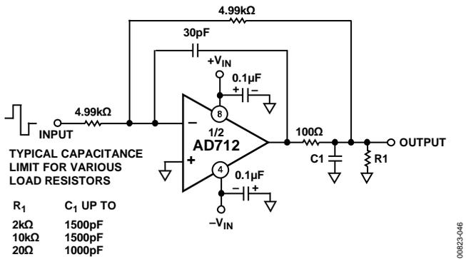
Figure 46. Circuit for Driving a Large Capacitive Load
