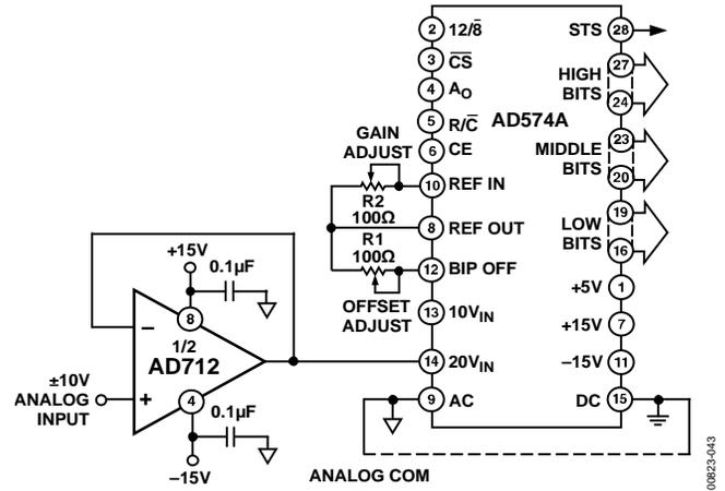
Figure 43. AD712 as an ADC Unity-Gain Buffer
