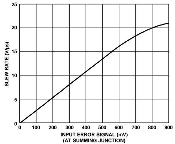
Figure 19. Slew Rate vs. Input Error Signal
