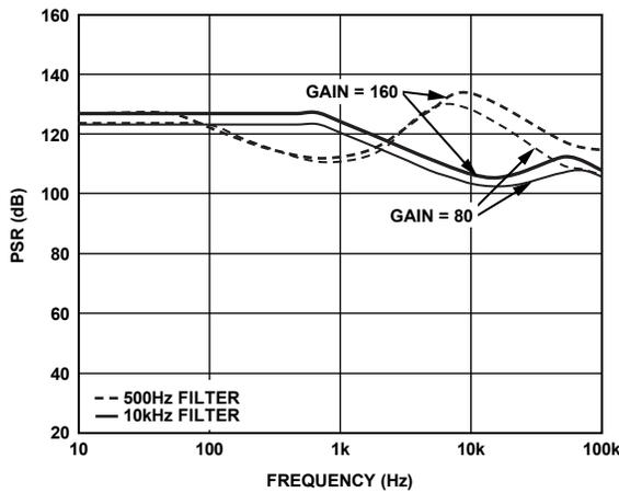
Figure 12. Power Supply Rejection (PSR) vs. Frequency
