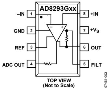
Figure 3. Pin Configuration
