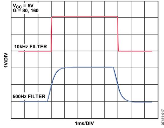
Figure 17. Large Signal Step Response
