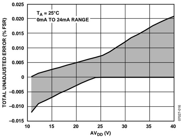
Figure 20. Total Unadjusted Error vs.  $AV_{DD}$ , External  $R_{SET}$
