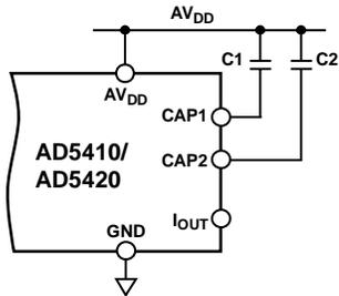
Figure 44. I<sub>out</sub> Filtering Capacitors
