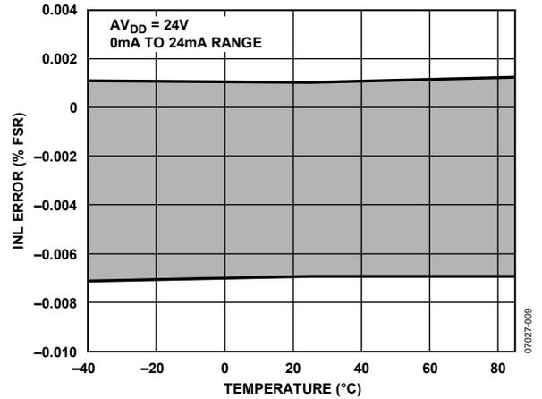
Figure 10. Integral Nonlinearity Error vs. Temperature, Internal RSET
