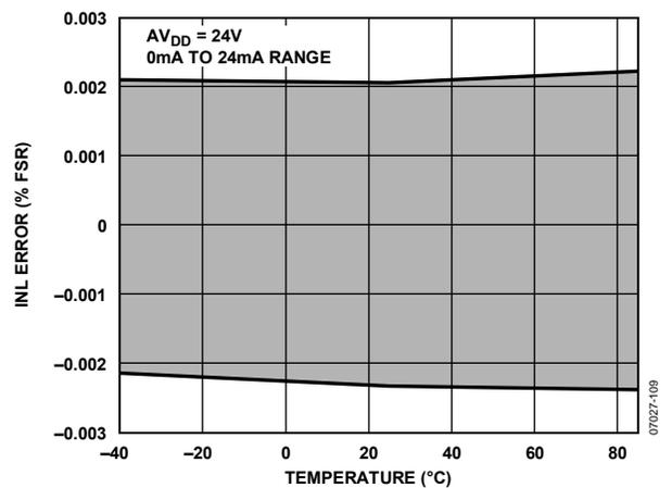
Figure 11. Integral Nonlinearity Error vs. Temperature, External RSET
