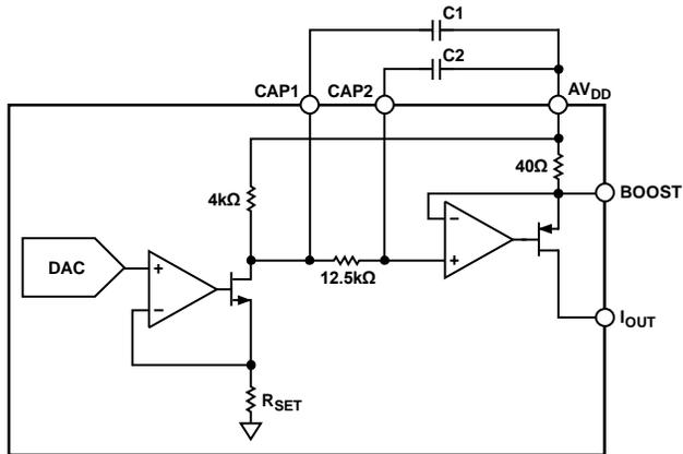
Figure 45. I<sub>out</sub> Filter Circuitry
