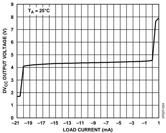
Figure 27.  $DV_{CC}$  Output Voltage vs. Load Current
