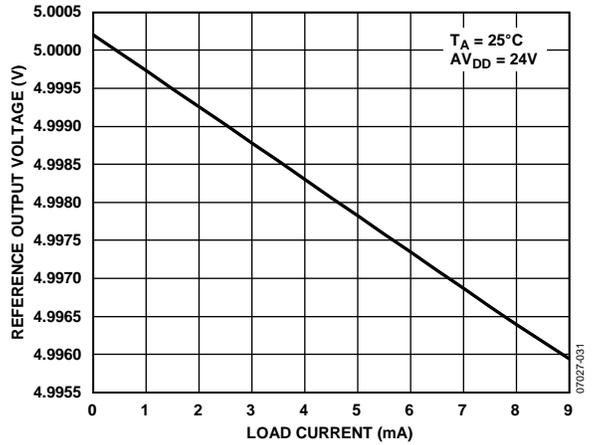
Figure 34. Reference Output Voltage vs. Load Current
