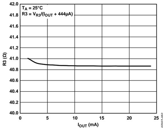
Figure 50. R3 Resistor Value vs. I<sub>OUT</sub>
