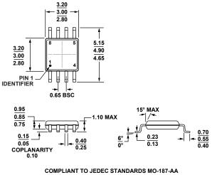
Figure 56. 8-Lead Mini Small Outline Package [MSOP] (RM-8) Dimensions shown in millimeters
