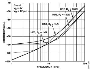
Figure 18. AD8007 Second and Third Harmonic Distortion vs. Frequency and RL
