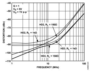
Figure 24. AD8008 Second and Third Harmonic Distortion vs. Frequency and Ru
