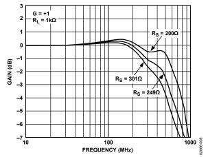
Figure 8. Small Signal Frequency Response for Various Rs Values
