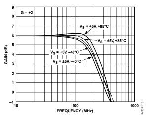
Figure 16. Small Signal Frequency Response over Temperature,  $V_S = \pm 5 V$ ,  $V_S = \pm 5 V$
