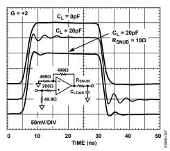
Figure 47. Small Signal Transient Response, Effect of Series Snub Resistor when Driving Capacitive Load
