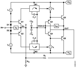
Figure 51. Simplified Schematic of AD8007
