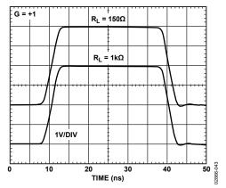
Figure 43. Large Signal Transient Response for  $R_L = 150 \Omega$ ,  $R_L = 1 k\Omega$
