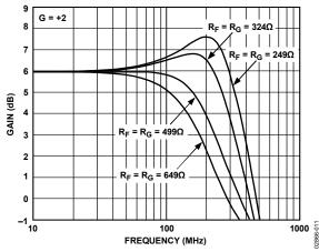
Figure 11. Small Signal Frequency Response for Various Feedback Resistors,  $R_c = R_c$
