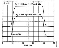
Figure 45. Small Signal Transient Response for  $R_L = 150 \Omega$ ,  $R_L = 1 k\Omega$  and  $V_S = \pm 5 V$ ,  $V_S = \pm 5 V$
