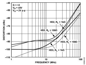
Figure 22. AD8007 Second and Third Harmonic Distortion vs. Frequency and R<sub>L</sub>
