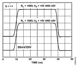
Figure 42. Small Signal Transient Response for  $R_L = 150 \,\Omega$ ,  $R_L = 1 \,k\Omega$  and  $V_S = \pm 5 \,V$
