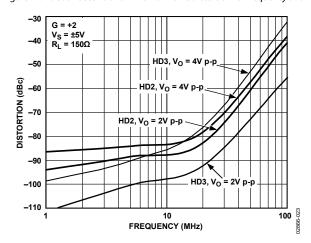
Figure 23. AD8007 Second and Third Harmonic Distortion vs. Frequency and  $V_{\rm O}$
