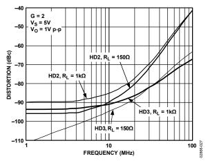
Figure 27. AD8008 Second and Third Harmonic Distortion vs. Frequency and RL
