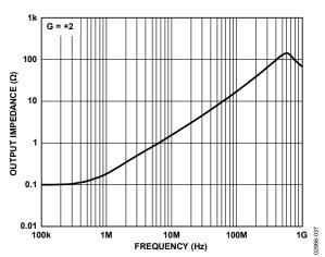
Figure 37. Output Impedance vs. Frequency
