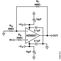
Figure 53. High Frequency Capacitors Returned to Ground at a Single Point (Recommended)
