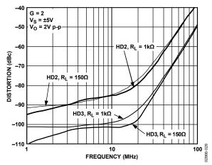
Figure 28. AD8008 Second and Third Harmonic Distortion vs. Frequency and RL
