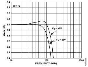
Figure 9. 0.1 dB Gain Flatness;  $V_S = \pm 5$ ,  $V_S = \pm 5$  V
