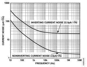
Figure 39. Input Current Noise vs. Frequency
