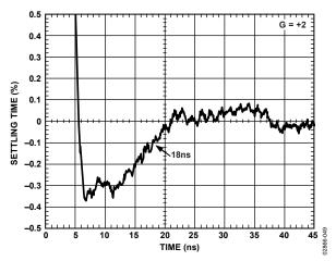
Figure 49. 0.1% Settling Time, 2 V Step
