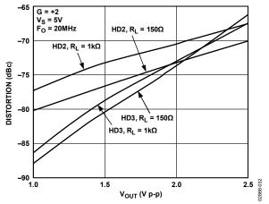
Figure 32. AD8008 Second and Third Harmonic Distortion vs.  $V_{\text{OUT}}$  and  $R_L$
