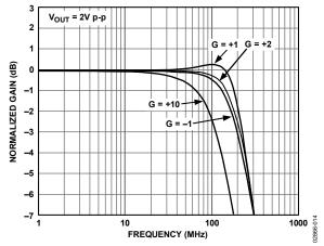
Figure 14. Large Signal Frequency Response for Various Gains
