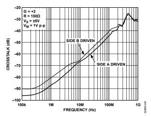
Figure 40. AD8008 Crosstalk vs. Frequency (Output to Output)
