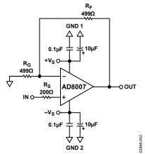
Figure 52. High Frequency Capacitors Returned to Physically Separate Grounds (Not Recommended)
