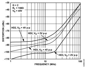
Figure 29. AD8008 Second and Third Harmonic Distortion vs. Frequency and  $V_0$
