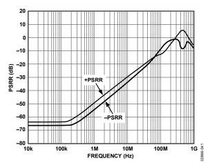
Figure 41. PSRR vs. Frequency
