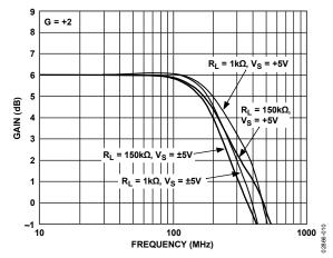
Figure 10. Small Signal Frequency Response for V<sub>S</sub> and R<sub>L</sub>
