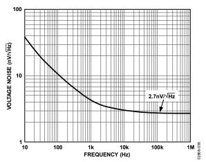
Figure 36. Input Voltage Noise vs. Frequency
