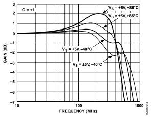
Figure 13. Small Signal Frequency Response over Temperature,  $V_S = \pm 5 V$ ,  $V_S = \pm 5 V$
