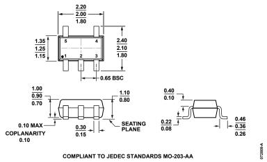
Figure 57. 5-Lead Thin Shrink Small Outline Transistor Package [SC70] (KS-5) Dimensions shown in millimeters
