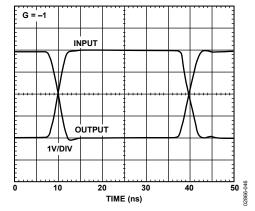
Figure 46. Large Signal Transient Response, G = -1,  $R_L = 150 \Omega$
