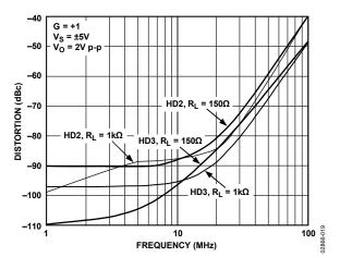
Figure 19. AD8007 Second and Third Harmonic Distortion vs. Frequency and RL
